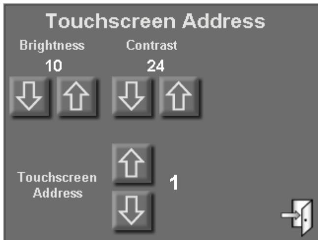
This page allows the installer to adjust the brightness and contrast of the touchscreen and assign the touchscreen address.
